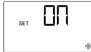
Fig.16 Ventilation function is on
