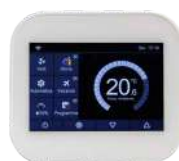
NPM/A1 - 010- Brushless Digital Wall-Mounted Controller 230V + 0-10 V + 2/4-pipe. 3.5-inch TFT colour touchscreen. Dry contact for window sensor. Input for water sensor. Weekly programming + Wi-Fi. (requires a Ø60x40mm flush-mounted box, not included) Compatible with the 761080 square flush-mounted box (75x75x42mm), not included
