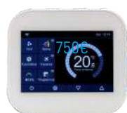
NPM/A1 - 230V Digital Wall-Mounted Controller + 3 speeds + 2/4 pipes. 3.5-inch TFT colour touchscreen. Dry contact for window sensor. Input for water sensor. Weekly programming + Wi-Fi. (requires a Ø60x40mm flush-mounted box, not included) Compatible with the 761080 square flush-mounted box (75x75x42mm), not included
