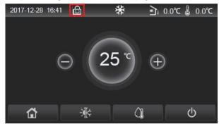
In this case, the control panel is locked and my any touch operation does not work. By touching for six seconds, the control panel will be unlocked and touch operation will work. However, the setting of "**Child Lock**" will remain to be "**ON**", and if there is no any operation in 30 seconds, the control panel will be locked again.
