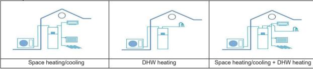
There are five basic working modes, including space cooling, space heating, domestic water heating, space cooling plus domestic water heating, and space heating plus domestic water heating.
