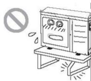
If damaged, it may cause fall of the unit and injury of people. When there is not water in water tank, never power the unit on to run.
