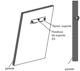
Step3: Attaching indoor unit to the wall.
