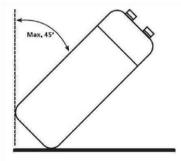
ATTENTION: DUE TO THE HIGH CENTER OF GRAVITY, LOW OVERTURNING MOMENT, THE UNIT MUST BE SECURED AGAINST TIPPING OVER.
