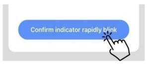
Notes: when the icon of set flashes quickly, it mean the controller is in the Wi-Fi mode. When it flashes slowly, it means the controller is connecting with the App. During the connection, if the icon of set is extinguished, it means the App connection with the unit is finished.
