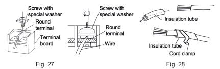
(3). How to fix connection cord and power cord by cord clamp
